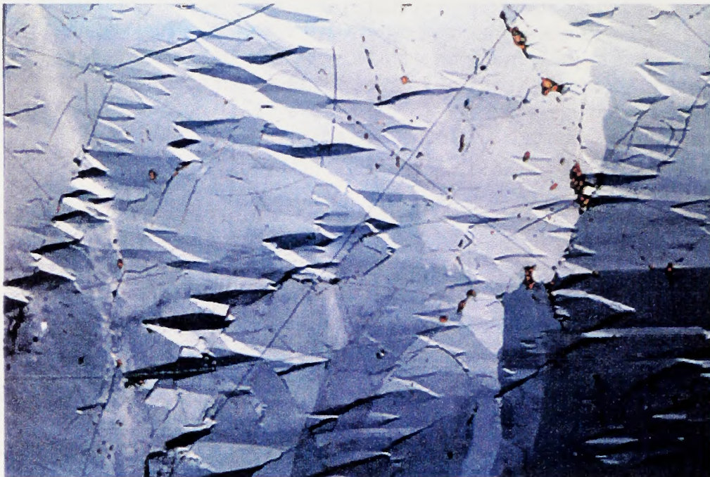
Fig.26: Photomicrograph of euhedral stibnite (antimonite) mineralization. Reflected light on polished surface, oil imersion, crossed-polars. Bottom edge of picture is 0.7 mm in length.
